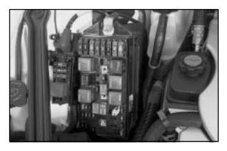
Some fuses are in the underhood electrical center on the passenger's side of the engine compartment.
