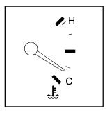
You have a gage that shows the engine coolant temperature. If the gage moves into the red area, your engine is too hot. That reading means the same thing as the warning light. It means that your engine coolant has overheated. If you have been operating your vehicle under normal driving conditions, you should pull off the road, stop your vehicle and turn off the engine as soon as possible.
