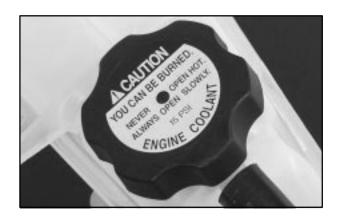
When the engine is cold, the coolant level should be at or above the FULL COLD mark on the coolant surge tank. If it isn't, you may have a leak in the radiator hoses, heater hoses, radiator, water pump or somewhere else in the cooling system.
