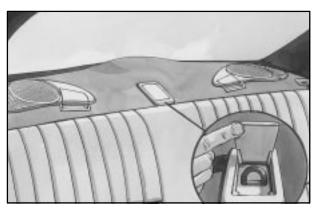
Anchor the top strap to this bracket. Once you have the top strap anchored, you'll be ready to secure the child restraint itself.
