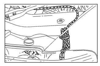
In very cold weather, 0°F (-18°C) or colder, the engine coolant heater can help. You'll get easier starting and better fuel economy during engine warm-up. Usually, the coolant heater should be plugged in a minimum of four hours prior to starting your vehicle.
