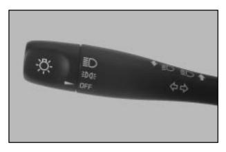
The lamp controls are located on the multifunction lever on the left of the steering wheel. They control these systems:
