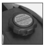
The power steering fluid reservoir is toward the middle of the engine compartment, on the passenger's side.
