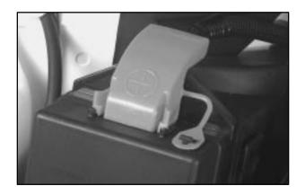
To uncover the remote positive (+) terminal, squeeze the sides of the red plastic cap and pull the cap toward you.
