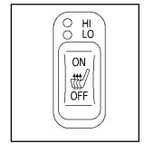
If your vehicle is equipped with this feature, both the driver's and passenger's heated seat switches are located on the instrument panel near the comfort controls. The driver's switch is on the left, and the passenger's on the right.
