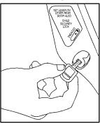
Your vehicle is equipped with rear door security locks that help prevent passengers from opening the rear doors of your vehicle from the inside.
