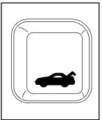
Press the button on the left side of the instrument panel to unlock the trunk from inside your vehicle. Your vehicle must be in PARK (P).
