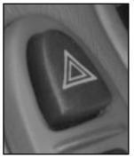
Press the switch located on your instrument panel to make your front and rear turn signal lamps flash on and off. Your hazard warning flashers work no matter what position your key is in, and even if the key isn't in.
