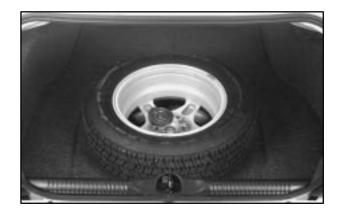
When storing a full-size tire, you must use the extension to help avoid wheel surface damage. Use the extension and protector/guide located in the foam holder. To store a full-size tire, place the tire in the trunk with the valve stem facing down and the protector/guide through a wheel bolt hole. Remove the protector and attach the retainer securely. When reinstalling the compact spare, put the protector/guide back in the foam holder. Store the cover as far forward as possible.
