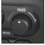
The PASS knob adjusts the air temperature on the passenger's side so it is warmer or cooler than the temperature set by the driver.
