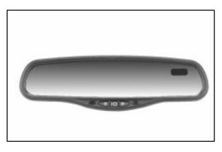
This mirror automatically changes to reduce glare from headlamps behind you. A time delay feature prevents rapid changing from the day to night positions while driving under lights and through traffic.
