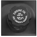
The engine oil fill cap is located toward the front of the engine compartment near the yellow looped engine oil dipstick.
