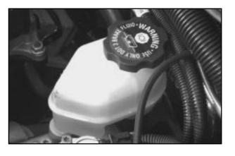
Your brake master cylinder reservoir is on the driver's side of the engine compartment. It is filled with DOT-3 brake fluid.
