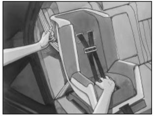
• If your vehicle has the child restraint locking feature on the shoulder belt retractor, pull the rest of the shoulder belt all the way out of the retractor to set the lock.
