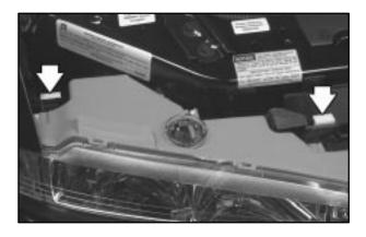
2. Pull straight up on the two headlamp retainers to release the assembly locator tabs and take the retainers off. At the same time, hold the headlamp assembly in position by applying a little pressure against the headlamp lens. This prevents the lamp from falling out.
