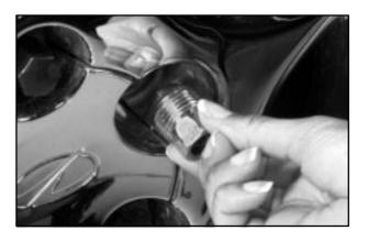
1. Using the wheel wrench, remove the plastic caps and loosen all of the wheel nuts. Don't remove them yet.
