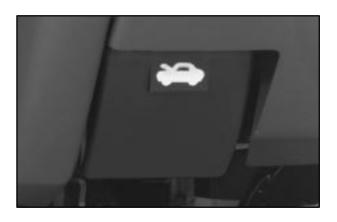
To open the hood, first pull the handle inside the vehicle. It is located below the instrument panel on the driver's side.
