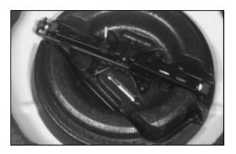
Turn the nut holding the jack counterclockwise and remove it. Then remove the jack and wrench.
