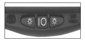
The mirror includes two map lamps, an automatic dimming function and an eight-point compass display in the upper corner of the mirror face. When the compass display is turned on, the compass automatically calibrates as the vehicle is driven.
