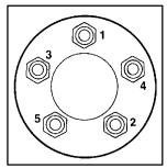
8. Tighten the wheel nuts firmly in a crisscross sequence as shown.
