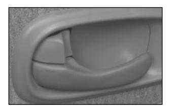
The rear doors do not have power door lock switches. The manual lever on each front and rear door works only on that door's lock. It won't lock or unlock all the doors. Push the manual lever rearward to unlock and forward to lock.
