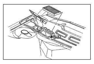
The passenger compartment air filter is located underneath the hood just below the windshield wiper arm on the passenger's side of the vehicle (underneath the air inlet grille).
