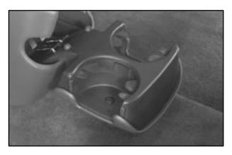
The cupholders are located in the rear of the front console. Pull down to use the cupholders.
