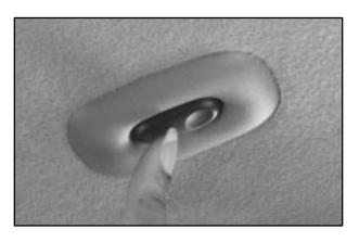
To open the power sunroof, press the rear of the switch once and the power sunroof will fully open. This is the express-open feature. During operation, press the switch again to stop the power sunroof at a desired position.
