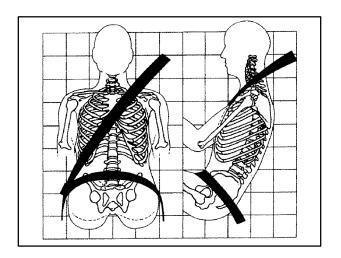
The lap part of the belt should be worn low and snug on the hips, just touching the thighs. In a crash, this applies force to the strong pelvic bones. And you'd be less likely to slide under the lap belt. If you slid under it, the belt would apply force at your abdomen. This could cause serious or even fatal injuries. The shoulder belt should go over the shoulder and across the chest. These parts of the body are best able to take belt restraining forces.
