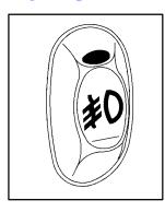
To turn the fog lamps on, press the top of the fog lamp switch located on the left side of the instrument panel.
