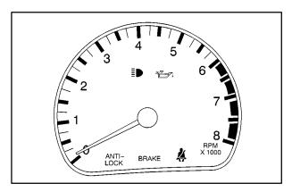
The tachometer displays the engine speed in thousands of revolutions per minute (rpm).
