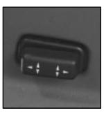
This switch is designed to imitate the movements of your seat cushion. It is located on the left side of the driver's or the right side of the passenger's seat cushion.
