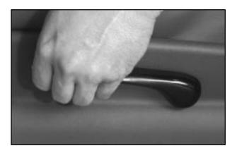
This lever is located on the left side of the driver's or the right side of the passenger's seat cushion. Lift the lever to release the seatback, then move the seatback to where you want it. Release the lever to lock the seatback in place. Pull up on the lever without pushing on the seatback and the seatback will move forward.
