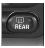
The rear window defogger uses a warming grid to remove fog from the rear window. Press the button to turn the defogger on. It will turn itself off after about 15 minutes (automatic control) or 10 minutes (manual control).
