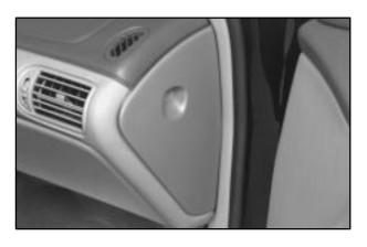
These fuses are located in a fuse block on the passenger's side of the instrument panel. Pull off the right side cover to expose the fuses.
