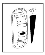
You can brighten or dim the instrument panel lights by turning the interior lamps thumbwheel.
