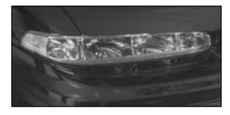
Your vehicle has a headlamp system equipped with horizontal and vertical aim indicators. The aim has been pre-set at the factory and should need no further adjustment. This is true even though your vertical and horizontal aim indicators may not fall exactly on the "0" (zero) marks on their scales.
