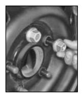
Reinstall the wheel nuts with the rounded end of the nuts toward the wheel. Tighten each nut by hand until the wheel is held against the hub.
