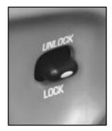
Press the power door lock switch located on the door near the handle to lock or unlock all doors.
