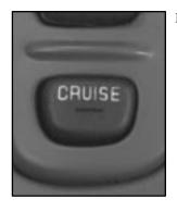
1. Press the CRUISE button on the right side of the instrument panel to turn it on. A light on the button will indicate that the system is on.
