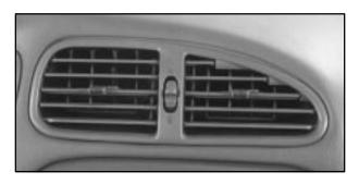
Adjust the direction of airflow by moving the vents. To completely shut off airflow to the outlet move the thumbwheel down. To open the outlet for airflow move the thumbwheel up.
