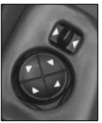
The power mirror control is located near the driver's window, on the armrest.
