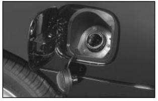
While refueling, let the cap hang by the tether below the fuel fill opening.
