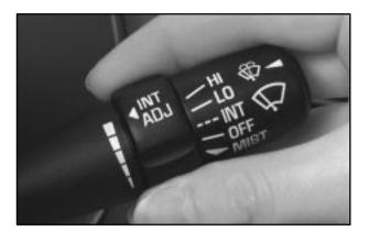
You can control the windshield wipers by moving the lever with the wiper symbol on it up or down. This lever is located on the right side of the steering wheel.
