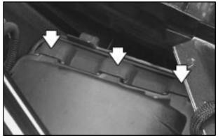
Be sure the tabs on the cover are inserted into the air box slots.
